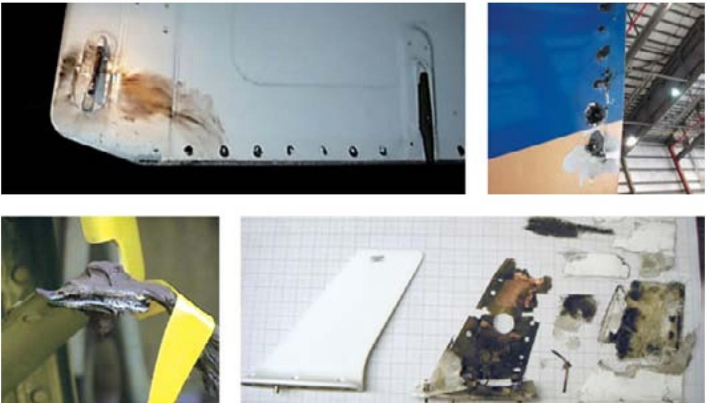
Because the airplane flies more than its own length during the time it takes a strike to begin and finish, the entry point will change as the flash reattaches to other spots aft of the initial entry point. Evidence of this is seen in strike inspections where multiple burns are seen along the airplane's fuselage (see fig. 6).
