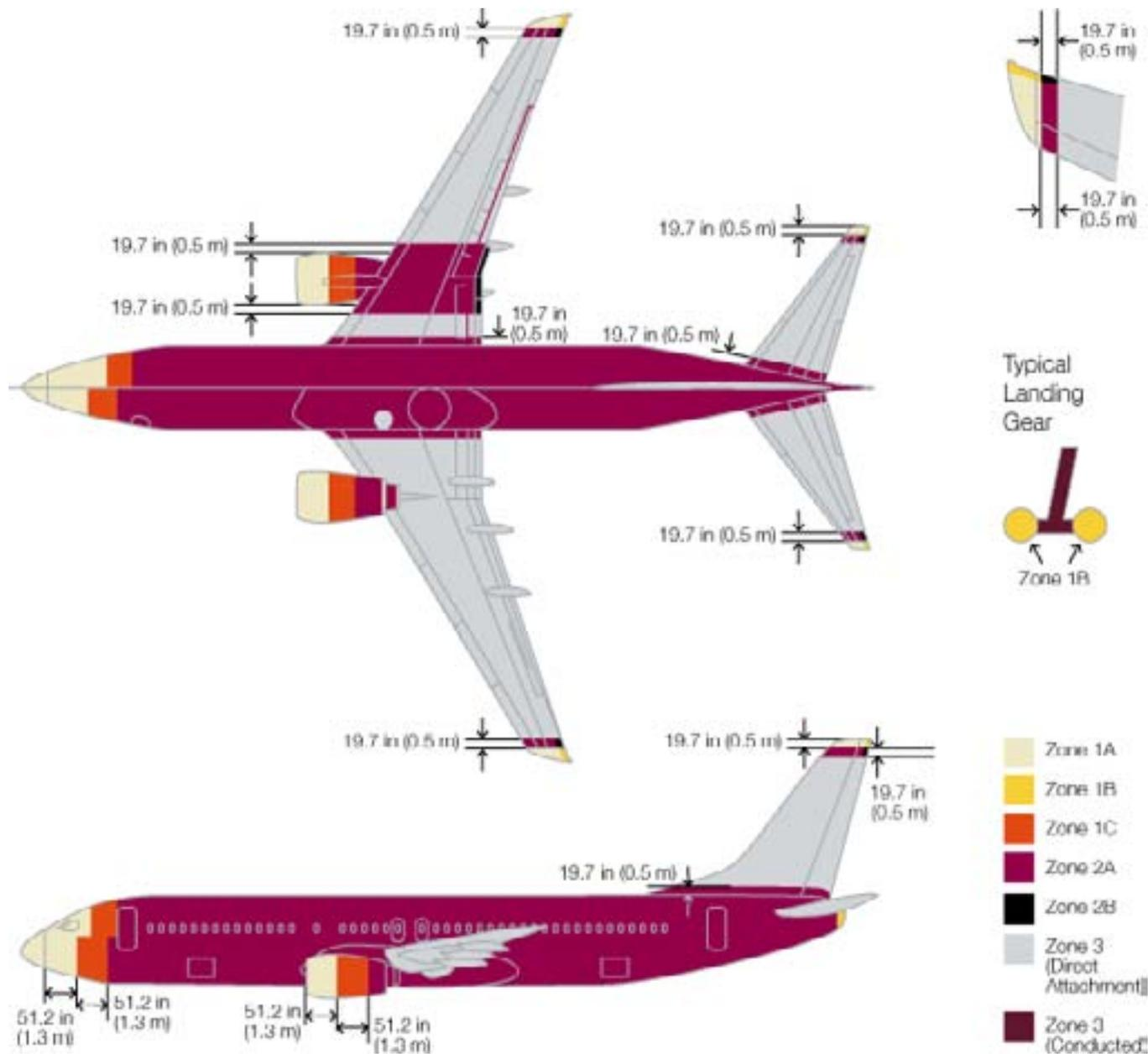
In Zone 2, an initial entry or exit point is a rare event, but in such a case, a lightning channel may be pushed back from an initial entry or exit point. As an example, the radome may be the area of an initial entry point, but the lightning channel may be pushed back along the fuselage aft of the radome by the forward motion of the airplane.
