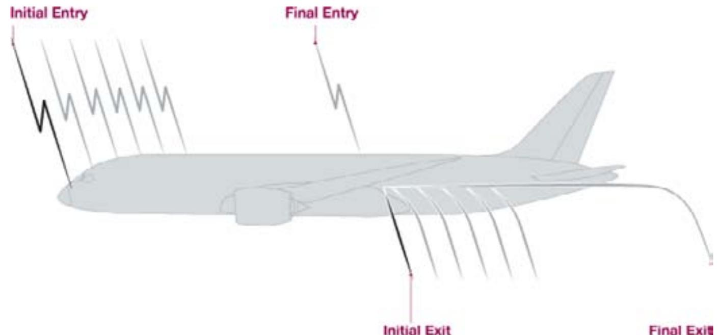
During the initial stages of a lightning strike on an airplane, a glow may be seen on the nose or wing tips caused by ionization of the air surrounding the leading edges or sharp points on the airplane's structure. This ionization is caused by an increase in the electromagnetic field density at those locations. In the next stage of the strike, a stepped leader may extend off the airplane from an ionized area seeking the large amount of lightning energy in a nearby cloud.
